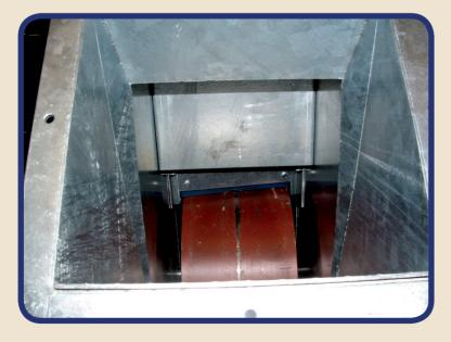
Solid crowned head drum as standard - boot drums slatted as standard with our configurations available depending on product requirements.
