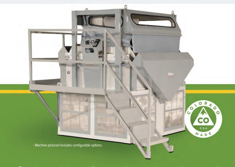
This maximum capacity destoner purifies your product by separating heavy materials such as glass, dirt, stones and metals from larger quantities of lighter material. Add value on a variety of products with the most precise destoner on the market — Oliver's legendary Maxi-Cap Destoner.
