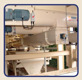
Standard diameters from 150mm to 1000mm. Larger diameters on request. Stainless steel / galvanised steel / mild steel powder coat painted construction options.
