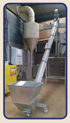
Standard diameters from 150mm to 1000mm. Larger diameters on request. Stainless steel / galvanised steel / mild steel powder coat painted construction options.
