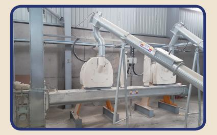
Can be inclined up to vertical. General conveying, intermediate outlets available.
