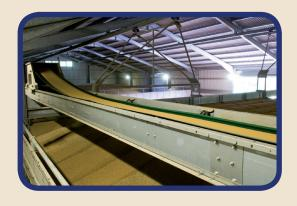
These designs give an exceptionally rigid construction, easily capable of spanning 6m building bays.
