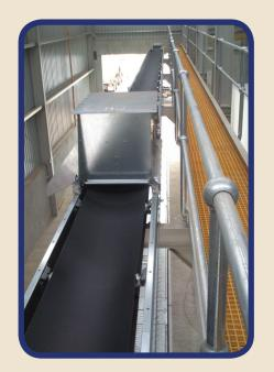
Capacities of up to 800tph based on wheat at 750kg/m<sup>3</sup>.
